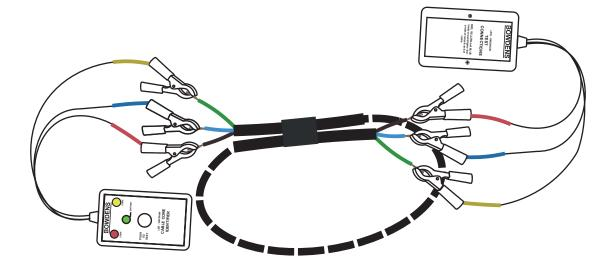
To test the CCI, connect the leads together and check the LED response.
