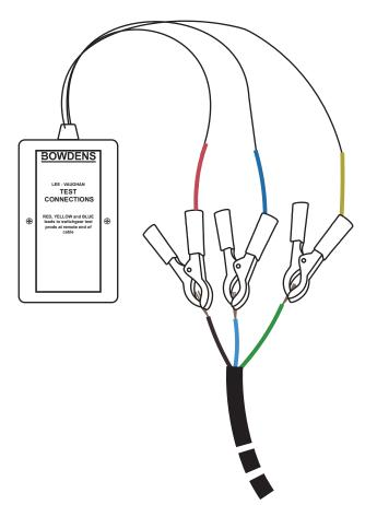
Connect the leads at the remote end in any order. Push the button on the Transmitter. In this example the red LED is on. The yellow LED is off. The green LED always lights. Now follow the instructions on the back of the Transmitter.
