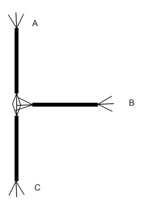
If the phases are correctly connected at both A & B then phase identification at C is valid using a receiver at either (not both) A and B.
