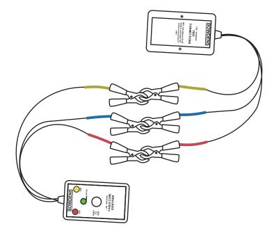
Note: Care must be taken if parallel circuits exist which may not be obvious from the test points. A cross between two phases on one of the parallel cables will not be identified, unless the circuits are tested individually.
