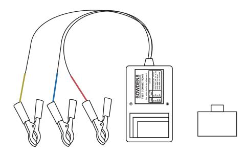
Push button on transmitter to carry out battery test. If green LED does not light, change the battery but only with an industrial capacity Alkaline PP3.
