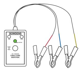
Connect the receiver leads to the switchgear prods or the connected cable end. If the colours do not match make a note of the relationship between the lead colours and the cable core colours.
