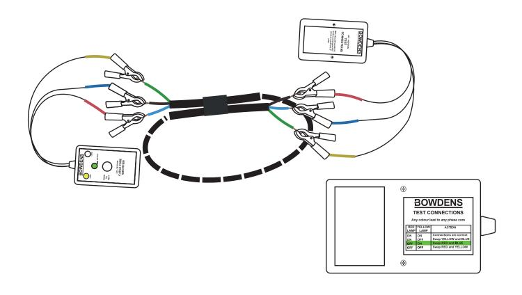
The instructions tell us to swap the red and blue leads. Press the button and both the red LED and the yellow LED are lit. This means the phase rotation is now correct.
