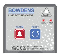
If the unit is not in alarm mode, pressing 'RESET' will test the battery. The two red LEDs will flash red just once if the battery is OK. Alternatively, the unit will flash the two red LEDs 10 times to signify that the battery is low.
