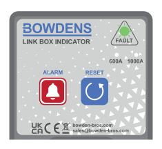
If the unit detects a fault above the set trip level the unit will enter the ALARM state by blinking the fault LED twice and thereafter blinking once every 10 seconds approximately. The unit will complete a timed reset after approximately six hours. (Operators can reset before this time by pressing the 'RESET' button).
