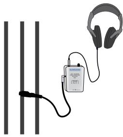
Where access to cables is very tight, the roving coil can be plugged into the side of the receiver and used to good effect.
