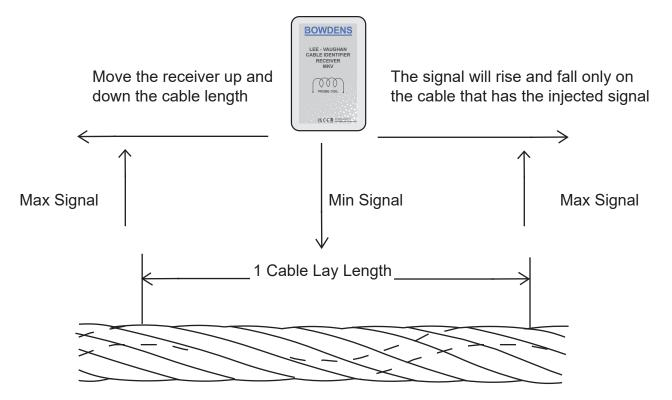
Adjacent cables may pick up a small amount of inducted signal, but the signal will not rise and fall, this will only happen with the target cable to which the transmitter is connected.
