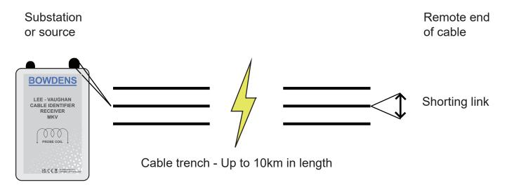
The signal in the headphones will rise and fall with the lay of the cores.
