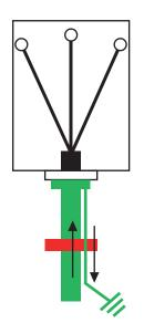
Traditional external cast resin C/T installation. Insulated gland at entry to cable box. An earth braid needs to be soldered to the earth termination and brought back through the C/T to cancel the earth fault flowing in the cable sheath.
