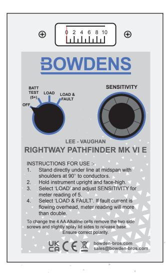
AN OVERHEAD LINE FAULT PASSAGE INDICATOR THAT WORKS IN CONJUNCTION WITH ARC SUPPRESSION COIL NETWORKS
