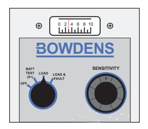
D) Turn the selector to 'Load + Fault' and observe the meter.
