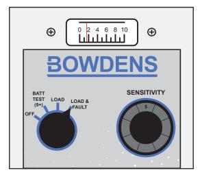
F) If the reading increases by a factor of two or more, there is fault current flowing and the fault lies further down the line.
