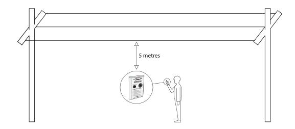
C) Turn the selector to 'Load' and adjust the sensitivity knob until the meter reading is five. If the Meter will not read five, leave sensitivity adjusted to maximum.
