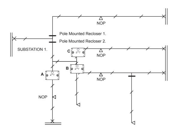
When the fault occurs PMAR two trips. The MK8 at C flags. The instruments at A and B do not trip. We know that the fault lies between the MK8 at C and the Normally Open Point (NOP).
