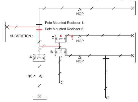
Trying to locate a fault due to a cracked insulator can be very difficult. The MK8's can be re-deployed down the main line a few poles apart to divide the network up into the smallest sections.
